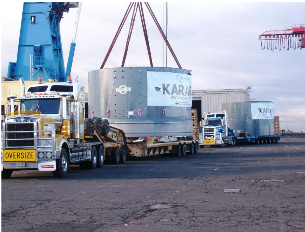
Figures 2: Completed Ball Mill shells being loaded for transport from Melbourne to Fremantle.
