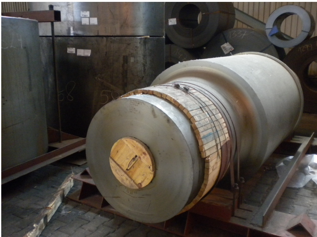
Figure 1: HPGRs under construction for the Karara Iron Ore Project.
